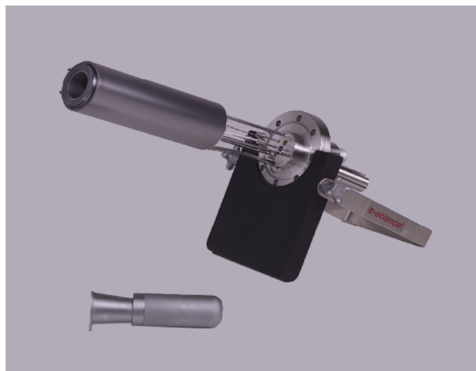
Fig. 1. The E-Science Titan effusion cell incorporates a two-piece graphite crucible that provides lower defect counts, improved uniformity, high capacity, reduced shutter transients, and a shorter conditioning time.
